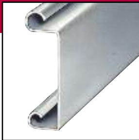
No. 14 —Flat-faced slat available in up to 18-gauge steel or up to 18-gauge stainless steel. Depth of crown: \frac{3}{4} ", 2\frac{1}{4} " on centers.
